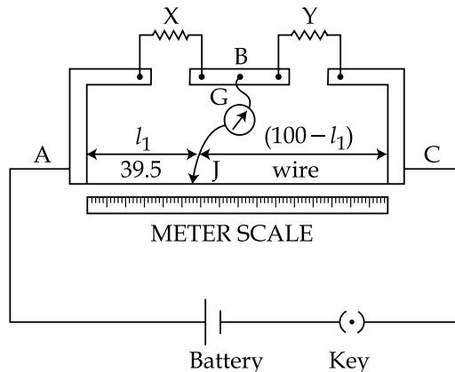
In a meter bridge, as shown in the figure, it is given that resistance  $Y = 12.5 \Omega$  and that the balance is obtained at a distance 39.5 cm from end A (by Jockey J). After interchanging the resistances X and Y, a new balance point is found at a distance  $l_2$  from end A. What are the values of X and  $l_2$ ?
