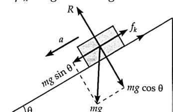
$$\begin{aligned}\therefore a &= g(\mu_k \cos \theta - \sin \theta) \\ &= g \left( \frac{1}{\sqrt{3}} \cos 30^\circ - \sin 30^\circ \right) \\ &= g \left( \frac{1}{\sqrt{3}} \cdot \frac{\sqrt{3}}{2} - \frac{1}{2} \right) = 0\end{aligned}$$
