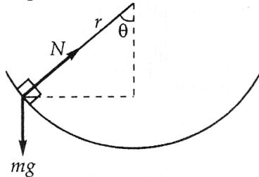
Resolving the forces along horizontal and vertical directions,
