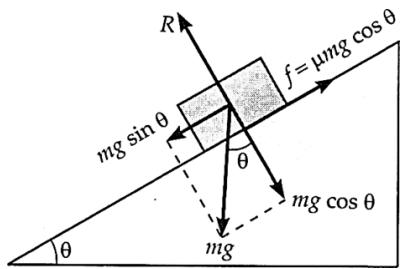
The contact force between the block and the inclined plane,
